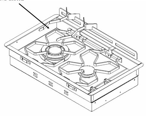
The cooking grate is designed to snap into place to ensure that it is level and to limit vibration.
